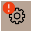
Fig. 155: The Service menu button with pending cleaning
