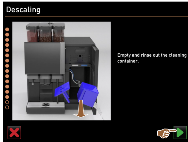
Fig. 248: Removing and emptying cleaning container
