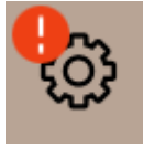
Fig. 135: The Service menu button with pending cleaning
