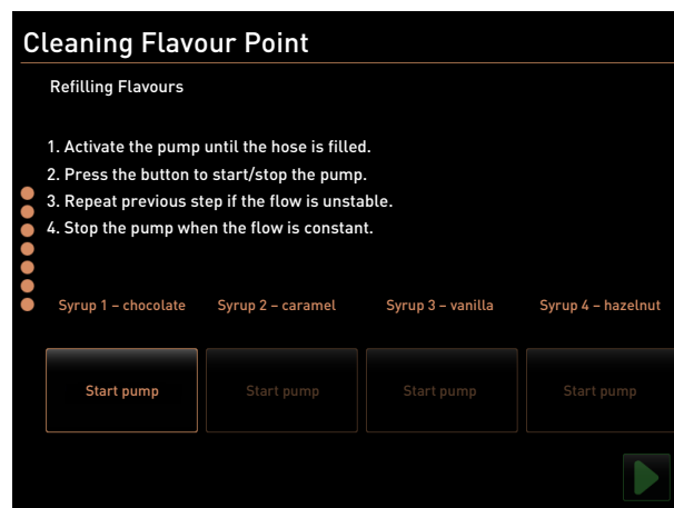
Fig. 185: Filling of syrup hoses
