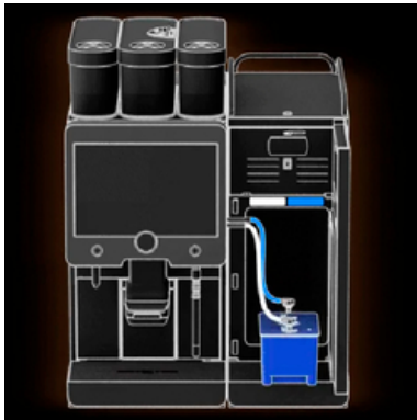
Figure: Placing the cleaning container in the cooling unit
