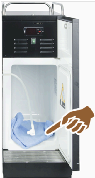
Figure: Cleaning cooling unit
