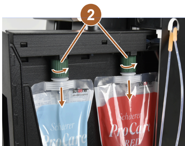
Figure: Removing cleaning bags
